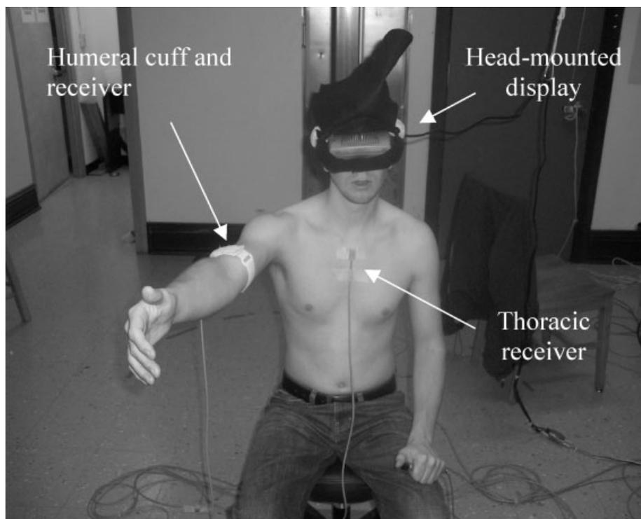
**Figure 2.** Photograph of experimental set-up showing sensors and head-mounted display.
